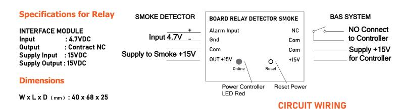
The smoke detector control box model BRDS-01 receives the signal. From smoke detectors Then convert signal into NO contact
